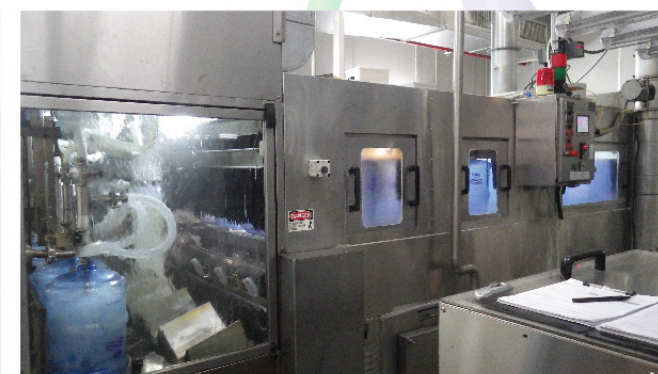
五加倫灌注機 Integrated Carboy washer / rinser / filler - improves the filling time to achieve a faster filling process
