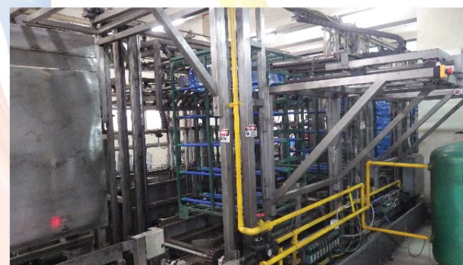
五加倫疊板機 Carboy Loader - new mechanical design improves the service life time and reduce downtime
