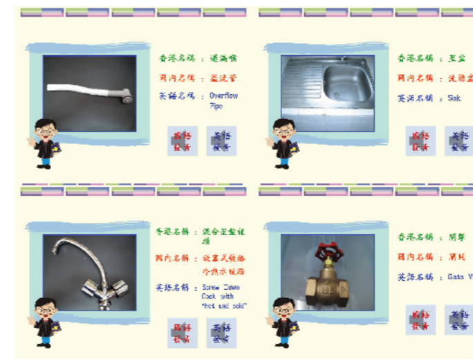
教學軟件提供室內潔具設施的正確名稱 Software teaching kit demonstrates the correct names of the sanitary wares and parts
