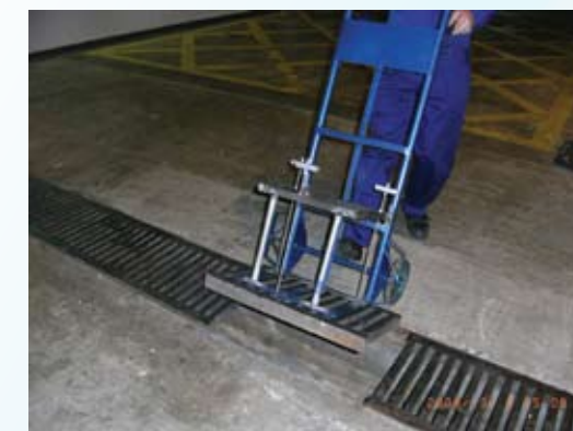
○ 有了「起排骨渠蓋車」的助力，揭渠蓋就輕鬆及安全得多了。 With the Smart Channel Cover Lifter, channel covers can be easily lifted up in an easier and safer manner.
