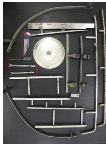
改善前需安裝 13 件零件及使用 9 件工具。 Thirteen parts and 9 tools are required for the changeover before the modification.
