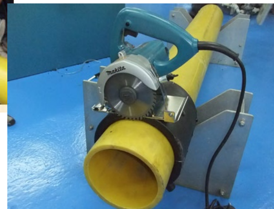
自行研製切割工具「套筒切管器」 Self-developed "Coupler-assisted Pipe Cutter"
