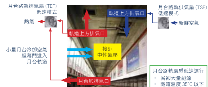
優化後機場快綫及東涌綫月台軌道氣流圖 Overview of the optimised Trackway Fans Air Flow at the platforms of AEL & TCL
