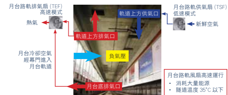
優化前機場快綫及東涌綫月台軌道氣流圖 Overview of the existing Trackway Fans Air Flow at the platforms of AEL & TCL
